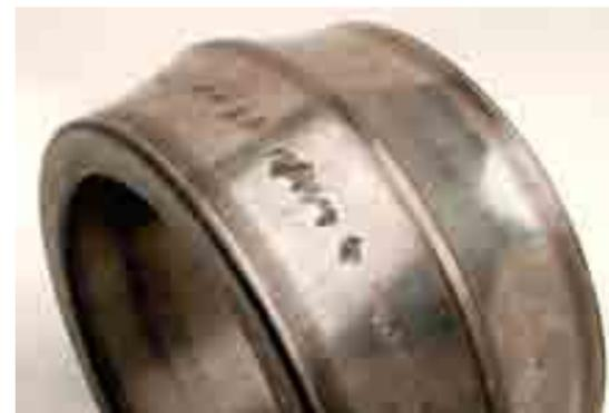
Disassembled bearing with spallings.
